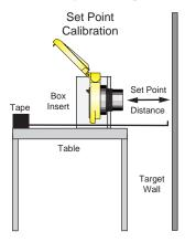
**D. Entering the CAL Mode:** To enter the CAL mode, you must first disable the calibration lock out feature. To do so, press and hold the SELECT button down. While holding the SELECT button, slide the RUN/CAL switch LEFT to the CAL position, and then release the SELECT button. At this point, all relay LEDs should be OFF.
