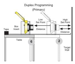
11. Position the switch at the desired HIGH HIGH set point distance defined as the air gap space between the transducer and the target.
