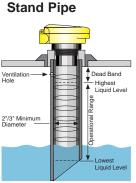
4. **Stand Pipe**: A stand pipe may be used to dampen turbulence or separate surface foam. Select a 2" or larger pipe for models LU75-5\_ \_ 5 and LU72-5\_ \_ 5. Select a 3" or larger pipe for models LU71-5\_ \_5 and LU73-5\_ \_5. The pipe length should run the measurement span. Cut a 45° notch at the bottom of the pipe and drill a 1/4" pressure equalization hole high in the dead band.
