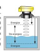
Automatic Fill or Empty: Programmed with two set points, the latched automatic fill or empty will control a pump or valve. When the level reaches the energize set point, the latching relay will energize, and remain energized until the level reaches the de-energize set point.
