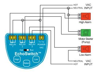
B. Wiring a LU7\_-58\_5 (12-28 VDC) to a Pump (Automatic Fill or Empty) and (Independent High and Low) Alarms
