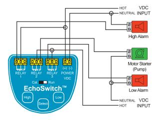
C. Wiring a LU7\_-50\_5 (95-250 VAC) to Pumps (Duplex or Alternating) and Alarm (Out of Bounds, High or Low)
