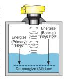
reaches the energize set point, the relays will alternate. If the level reaches the back-up energize set point, both relays will energize until the level reaches the de-energize set point. Alternation will automatically fill or empty the tank with two pumps switching after each cycle.
